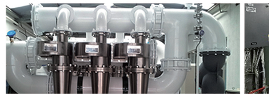
Ship Owner □ Germany (Peter Dohle) | Ship Type □ 38K BC Pump Capacity □ 700m 3 / h x 2 | Model □ BSKY 700 x 2 Skid Type Class □ LR
