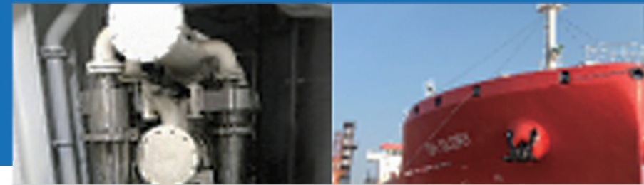
Ship Owner □ China | Ship Type □ 13K Chemical Tanker Pump Capacity □ 350m 3 / h x 2 | Model □ BSKY 700EX x 1 set Skid Type Class □ BV
